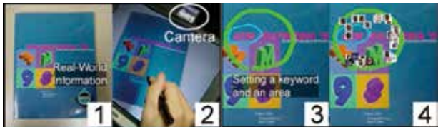
Figure 3: Combination with real-world information: Capturing real-world information as a picture (1, 2) and drawing a circle around the keyword brings up related information nodes (3, 4).
