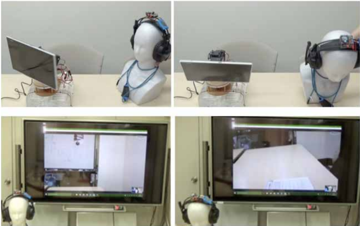
Figure 3. Basic Functions: The telepresence system moves depending on the remote user's head motion (top), and the viewpoint changes depending on the angle of the head if the remote user moves his/her head (bottom).
