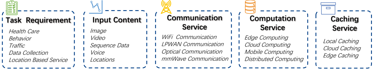
Fig. 1. Five categories are needed to realize IoT resource management framework: task requirement, input content, communication service, computation service and caching service.
