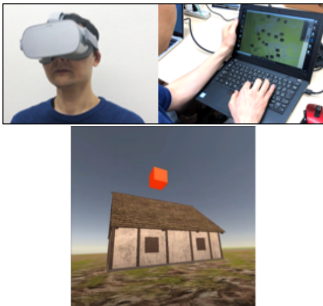
Fig. 4 Multiple devices and participants: directors can choose HMD or mobile devices to browse a shared virtual world (top left). Multiple participants share the same 3D scene (top right). When a director wears an HMD, his/her avatar does not appear (bottom).
